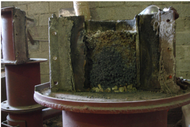
Fig. 6. View of part of the opened sinterpot with the formed sinter cake inside.
